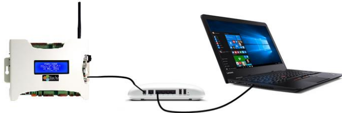
ECOM NANO and PC connection through Ethernet switch
