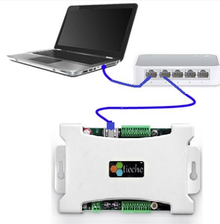
ECOM MICRO and PC connection via Ethernet switch
